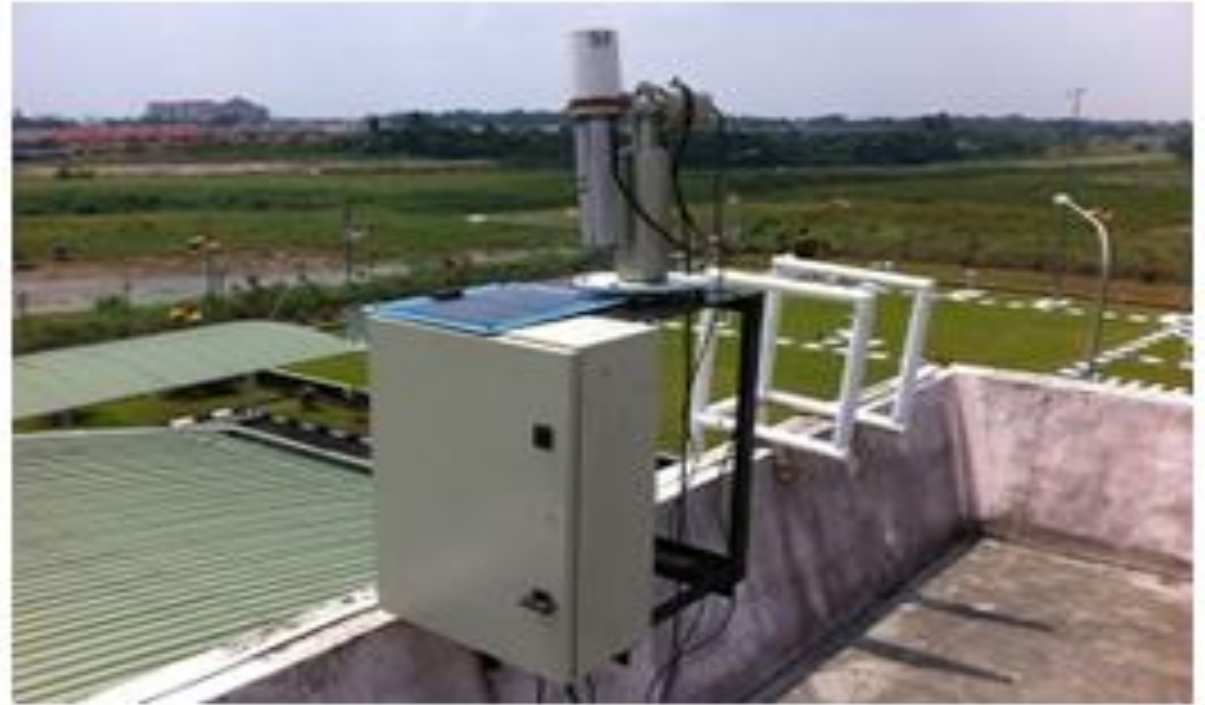
Figure 2: Location of AERONET Sun photometer at Observation Tower of Kuching Meteorological Station
